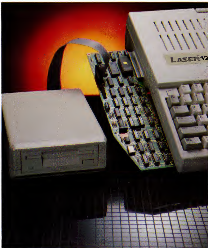
The Laser's Universal Disk Controller and 3½-inch drive—and the awkwardness of leaving cards in the side expansion slot.
